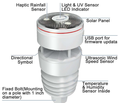
Figure 3 Sensor package assembly components
